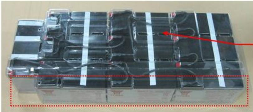
Batt. Wire should be placed in the slot of top cover.
